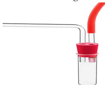
Figure 5. Hand-held mosquito aspirator (pooter) used for adult Aedes mosquito collection
